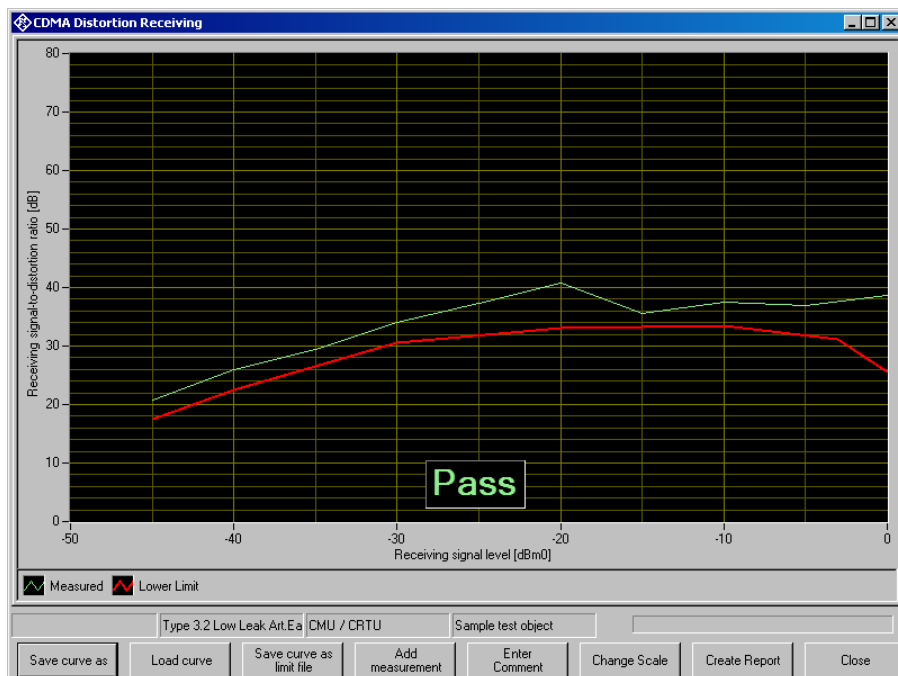
Fig. 26 Typical result of receiving distortion measurement
